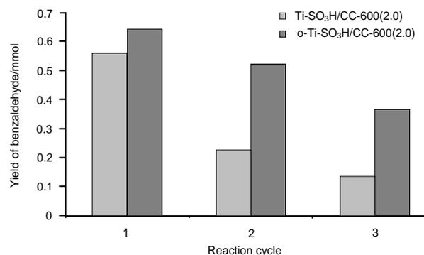
Figure 7. The capability to be reused of Ti-SO<sub>3</sub>H/CC600(2.0) and o-Ti-SO<sub>3</sub>H/CC600(2.0) in the oxidation of styrene (5 mmol), 30% H<sub>2</sub>O<sub>2</sub> (5 mmol) and catalyst (50 mg). The yield of benzaldehyde at room temperature for 20 h
