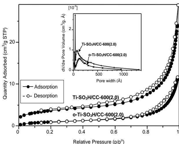
Figure 3. N<sub>2</sub> adsorption-desorption isotherms and BJH pore distribution of Ti-SO<sub>3</sub>H/CC-600(2.0) and o-Ti-SO<sub>3</sub>H/CC-600(2.0)
