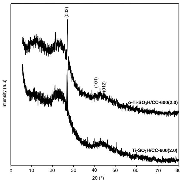
Figure 1. XRD pattern of Ti-SO<sub>3</sub>H/CC-600(2.0) and o-Ti-SO<sub>3</sub>H/CC-600(2.0)
