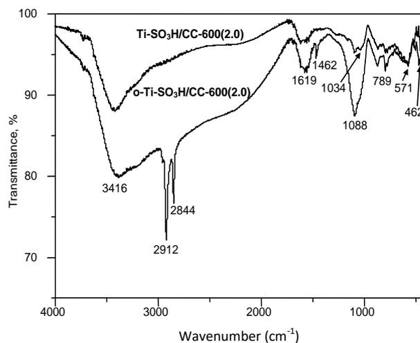
Figure 2. FTIR spectra of Ti-SO<sub>3</sub>H/CC-600(2.0) and o-Ti-SO<sub>3</sub>H/CC-600(2.0).
