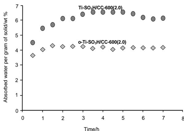
Figure 5. Water adsorption percentage for Ti-SO<sub>3</sub>H/CC-600(2.0), and o-Ti-SO<sub>3</sub>H/CC-600(2.0)
