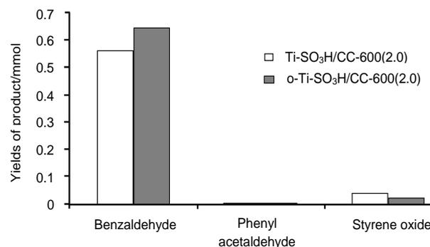
Figure 6. Comparison of catalytic activity of Ti-SO<sub>3</sub>H/CC600(2.0) and o-Ti-SO<sub>3</sub>H/CC600(2.0) in the oxidation of styrene (5 mmol), 30% H<sub>2</sub>O<sub>2</sub> (5 mmol) and catalyst (50 mg). The yield of product at room temperature for 20 h
