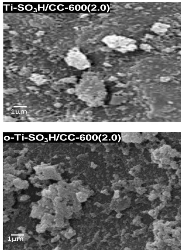
Figure 4. SEM images of Ti-SO<sub>3</sub>H/CC-600(2.0) and o-Ti-SO<sub>3</sub>H/CC-600(2.0)
